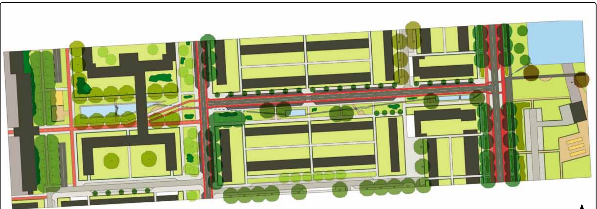
Design for a neighbourhood green strip with small scale water decoupling in Woenselse Heide
